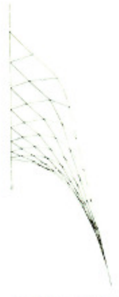
HALF OF EAST ELEVATION OF MAIN ARCH SHOWING BASIS OF STONE RIB PATTERN.
